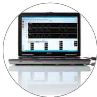
The advanced PC software enables on-line monitoring with wave forms, trends and numerical data.
